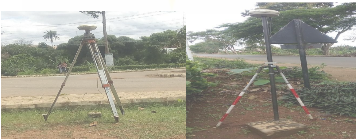
Figure 2: Static GNSS Observation. Base (fixed device on left), Rover (moved device on right)
