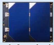
The module contains three channels for solar panels, for each axis of the satellite and a Li-Po battery with a capacity of 10.2 Wh. Each solar panel channel contains a DC-DC step-up converter that uses the MPPT algorithm to ensure maximum efficiency of converting solar energy into electricity and the output current of each power bus (5V, 3.3V, BCR).
