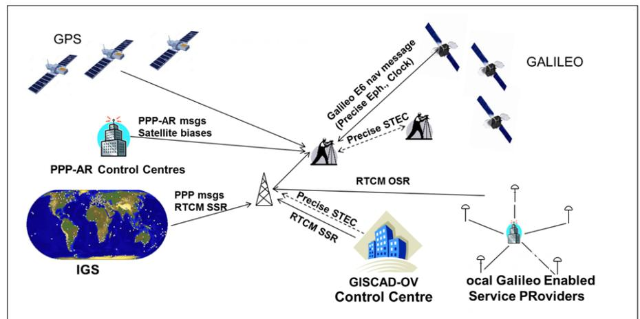
Fig. 1: Schematic overview of the GISCAD-OV architecture.
