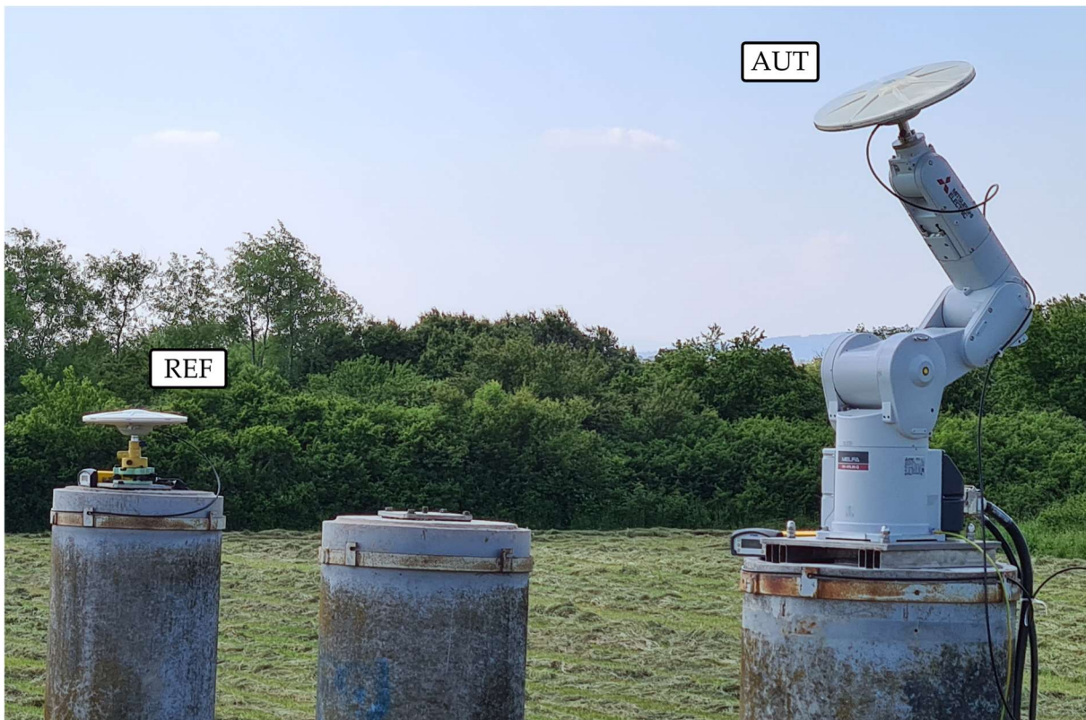
Figure 2. GNSS antenna calibration system during operation; REF – reference antenna, AUT – antenna-under-test (calibrated antenna).
